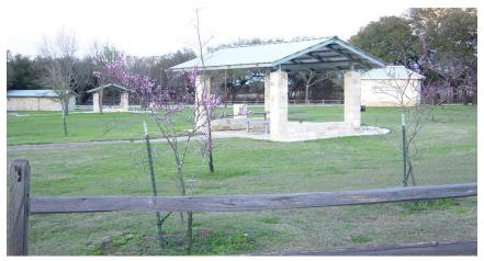
The storage building and monument sign can be seen beyond the picnic arbor. Picnic arbors were constructed using galvanized tube steel frames with limestone veneer and galvanized steel roofs.
